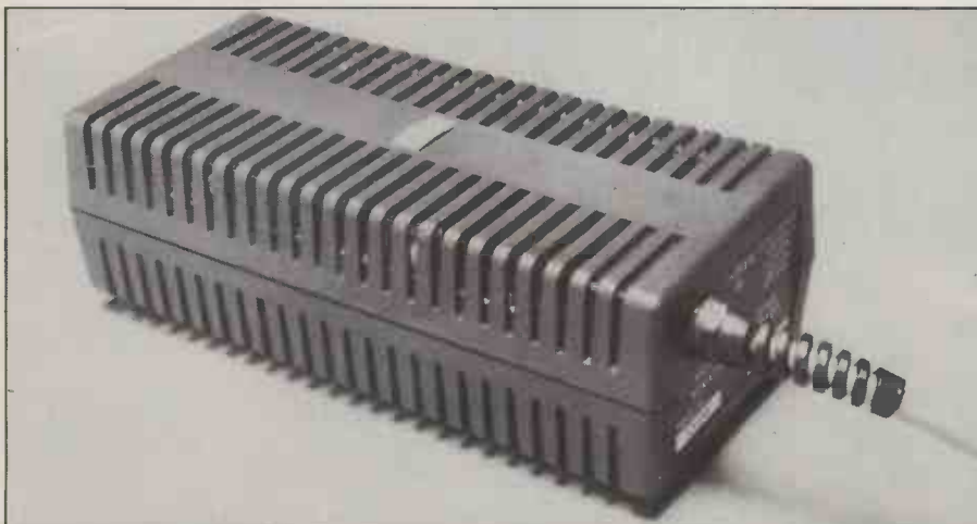
The main power supply is housed in its own well-ventilated casing.
